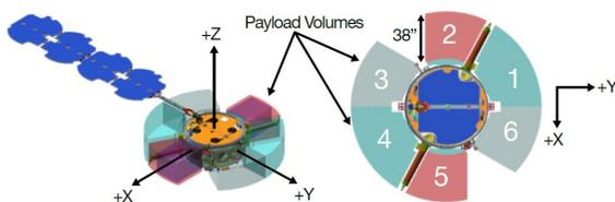
**Figure 3: LDPE accommodation wedges establishing virtual canister boundaries**
