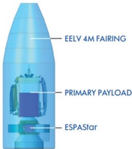
**Figure 2: ESPASStar bus illustrates the interfaces between a ‘primary’ payload and the need for ‘Do No Harm’ requirements<sup>2</sup>**
