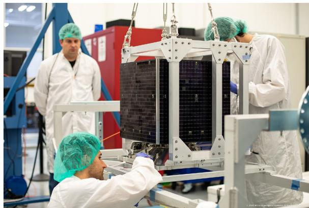
**Figure 4: Tetra-1 being assembled by Millennium Space Systems personnel<sup>4</sup>**
