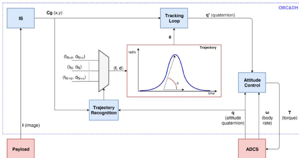
Figure 1: Autonomous Navigation System Functional Scheme
