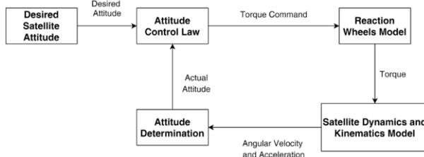
Figure 3: Attitude Controller Model Architecture
