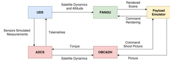
Figure 4: HIL Test Setup Diagram
