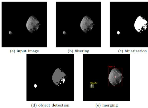
Figure 2: Example of the image processing pipeline
