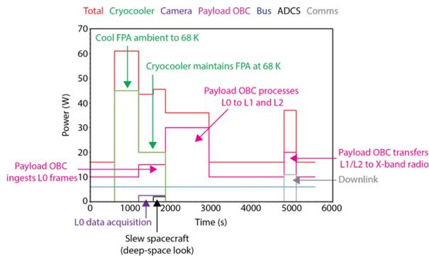
**Figure 7. Power consumption during data acquisition, processing and downlink, assuming all took place in a single orbit**
