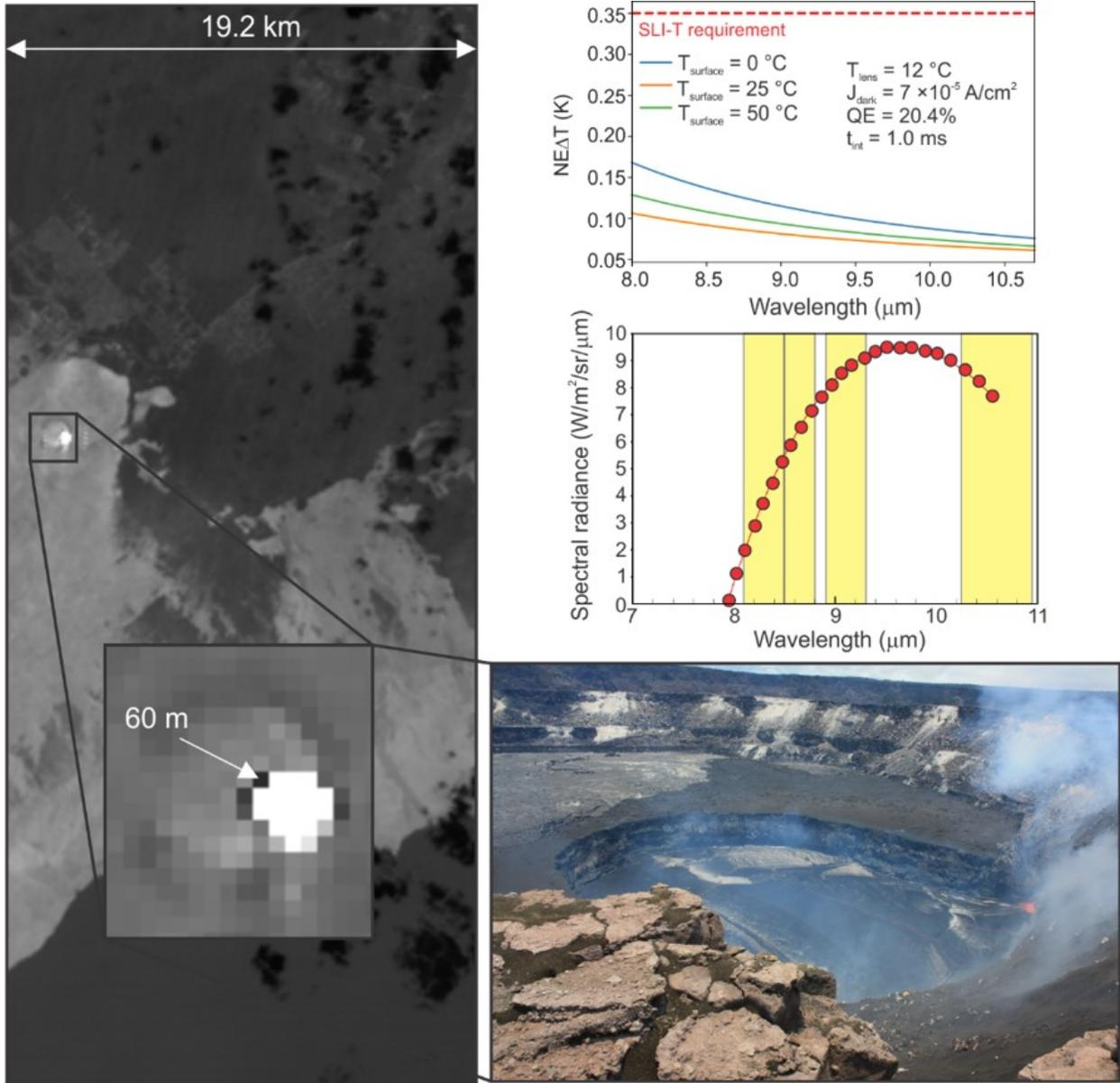
**Figure 2.** On the left, the approximate field of view (19 km swath) and spatial resolution of HyTI. On the right, NEAT predictions for HyTI, assuming a QE of 10%, with measured dark current (top). Illustration of the HyTI band count, compared to that of the Terra ASTER sensor (yellow bars).
