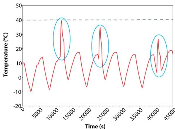
**Figure 4. Model prediction of the rejection temperature of the HyTI IDCA for a half day period, assuming relevant heat loads.**
