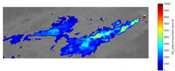
**Figure 5. PLSR-based retrievals of volcanic SO<sub>2</sub> from airborne MASTER data**
