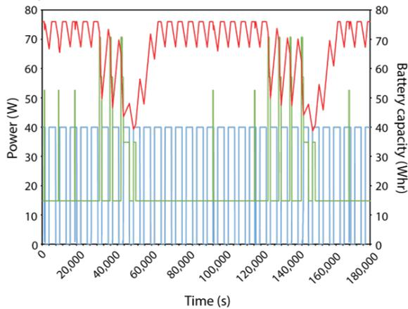
**Figure 6. Day-in-the-life power budget for HyTI baseline mission. Blue is power generation, green is power consumption, and red is battery capacity**
