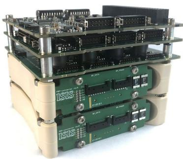
**Figure 7: ISISpace modular electronic power system used on Napa-1.**
