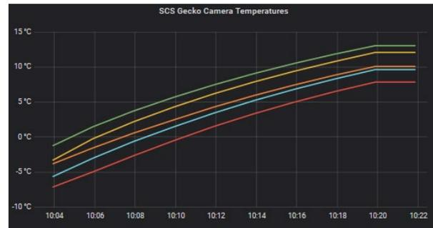
**Figure 16: Gecko camera temperatures reported right after enabling power.**
