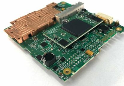
**Figure 8: ISISpace high-speed S-Band transmitter.**
