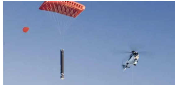
Figure 7: Depiction of Mid-Air Recovery by helicopter.
