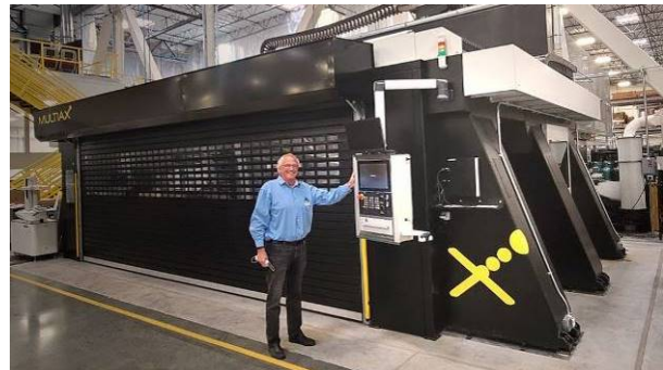
Figure 11: Virgin Orbit’s A-series composite milling machine by MultiAx America turbocharges an already-lean composites manufacturing process.
