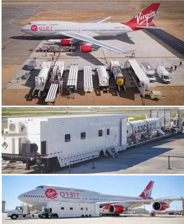
Figure 2: LauncherOne’s rapid-response mobile ground support trailers are globally transportable.
