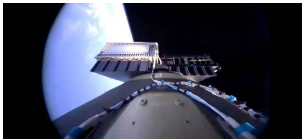
Figure 8: Camera footage of the VCLS Integrated Payload Stack (IPS) prior to deployment.
