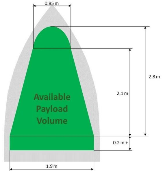
Figure 24: Geometry of Available Payload Volume
