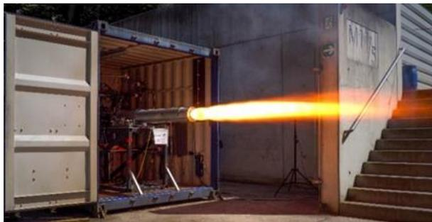
**Figure 6: Test of the 10 kN Demonstrator Motor**
