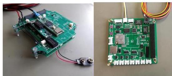
**Figure 13: On the left Measurement Unit Power and micro-controller unit, on the right the in-house built interface board for COTS flight controller**
