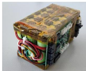
**Figure 14: Li-Ion battery pack assembled and ready to be tested together with its electrical control unit**
