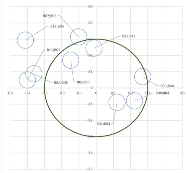
**Figure 6. Band to band x/y registration error for Sentinel 2B as measured by FLARE. Circle represents Sentinel mission requirement of < 0.3 pixels at >99.7% confidence.**
