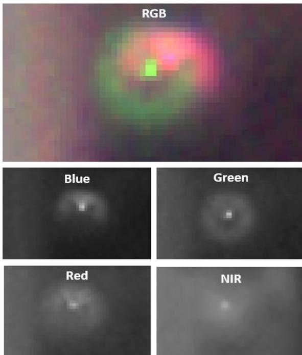
**Figure 9. Band-dependent registration and focusing errors identified during commissioning with FLARE. Once identified, these errors were rapidly corrected and subsequent imagery met all quality standards.**
