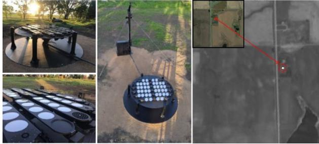
**Figure 1. FLARE node in Arlington, SD USA. Left, center: mirror array and instrumentation tower. Right: FLARE as observed by Sentinel 2B.**
