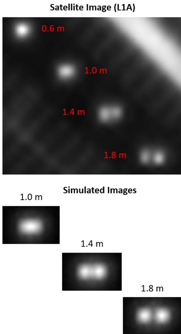
**Figure 7. Imagery of mirror point-pairs set at increasing distances, compared to simulated pairs using metrics generated from single points.**
