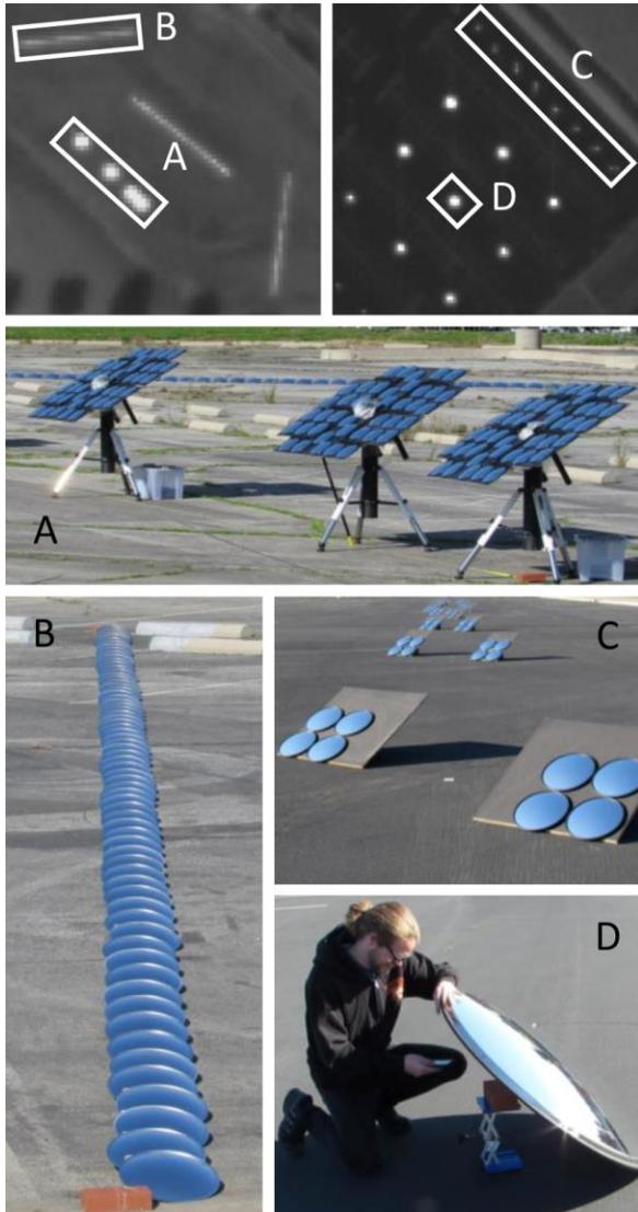
**Figure 2. FLARE campaign operations and target types used in rapid commissioning of small sats and verification of performance following orbital maneuvers.**
