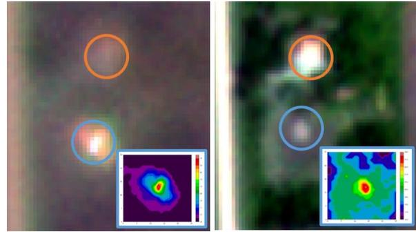
**Figure 10. Cross-track blur (left) and defocusing (right) artifacts identified with FLARE. Radiance from the sub-pixel mirror target (blue) was saturating, but can be observed in adjacent pixels. By contrast, a large, bright roof (orange) shows the spread of radiance from an extended target. This data can be utilized to improve telescope focusing and small-target radiometric retrieval techniques.**
