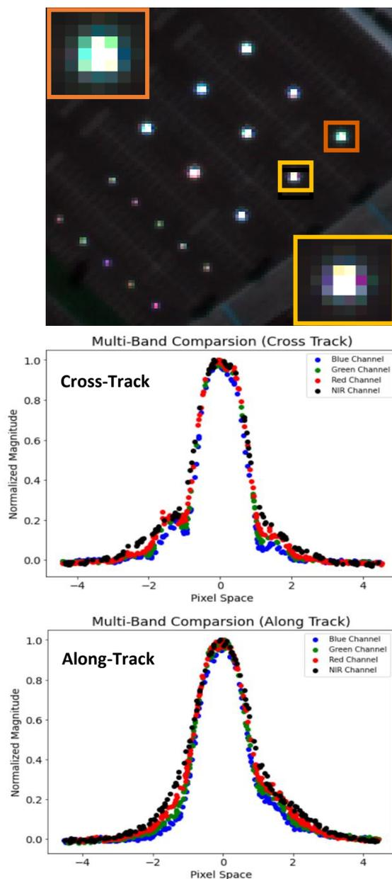
**Figure 8. Cross- and along-track response of the Point Response Function reveals good agreement between spectral bands.**
