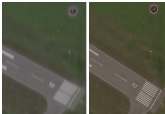
Figure 4: Direct comparison of image collections at a given scan rate with OIS disabled (left) and enabled (right).
