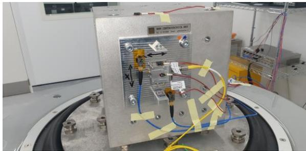
**Figure 2: First Generation Optics Module Under Vibration Testing**
