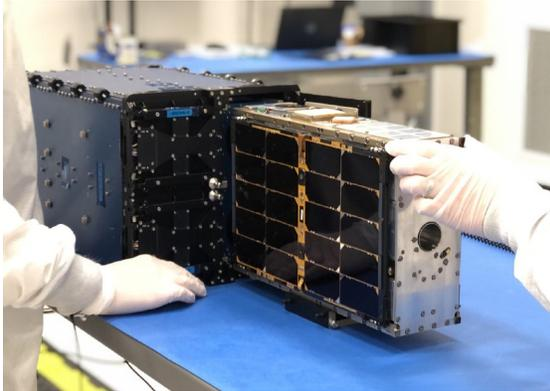
Figure 6: PTD-1 being loaded into the CubeSat deployer<sup>7</sup>
