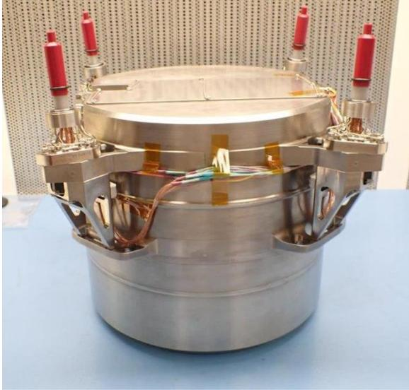
**Figure 9: Integrated Flight 1N Thrusters on IPS**
