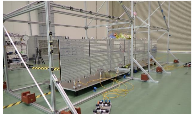
Figure 3 Successful deployment of the SAR antenna
