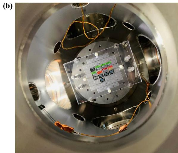
**Figure 2: Micro-SD cards under investigation. (a) Cards mounted on polycarbonate mount. Circle indicates the 8 cm diameter region of radiation exposure. (b) Bird's-eye view of cards and mount positioned in the SST chamber below the  $^{90}\text{Sr}$  source (retracted to allow view of samples).**
