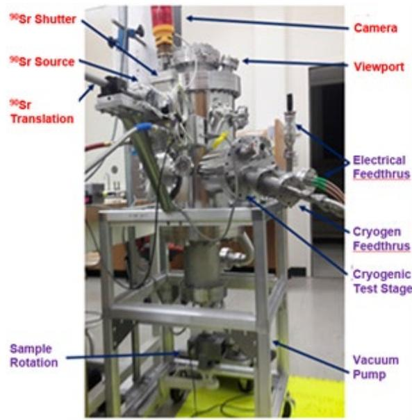
**Figure 3: Space Survivability Test (SST) chamber.**
