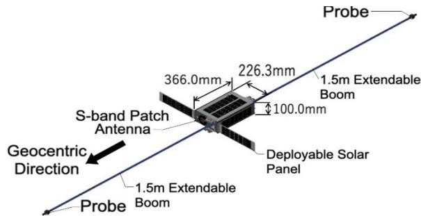
**Fig. 1: Prelude (Precursory electric field observation CubeSat demonstrator)**
