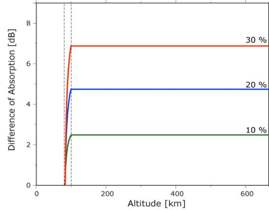
**Fig. 4: Difference in the amount of absorption of electromagnetic wave intensity due to the increase in electron density in the ionosphere**
