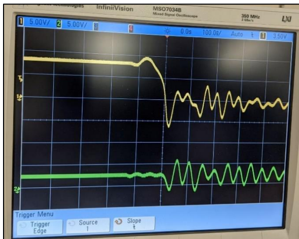
Figure 13: Switching Noise Waveform of Diode & Output Load
