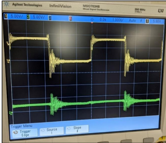
Figure 12: Voltage Waveform of Diode & Output Load
