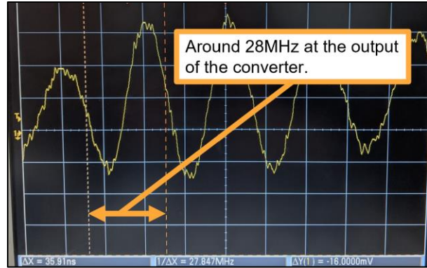
Figure 20: Output Noise of the Amazon Buck Converter Measured at Zero-Crossing
