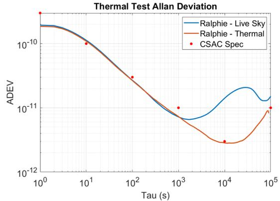
**Figure 10: Allan Deviation Using Receiver Estimated Clock Bias of *Ralphie* in Constant Temperature Hot Test**
