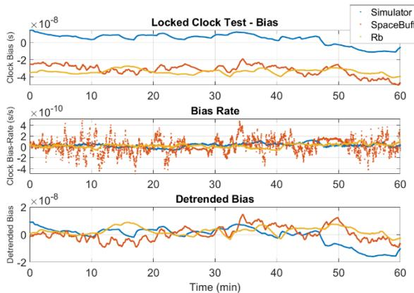
**Figure 6: Three Separate RF/GNSS Simulator Locked-Clock Tests Using a CSAC, Rb, and Spirent Simulator as External References**
