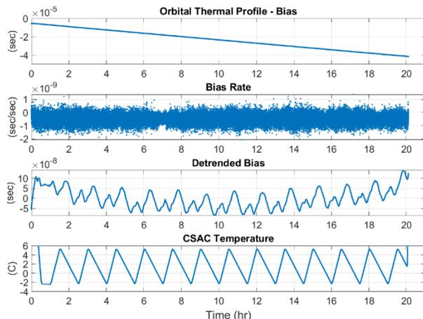
**Figure 12: Time series of bias, bias-rate, detrended bias, and temperature for CSAC orbital temperature profile test**
