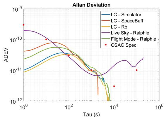
**Figure 8: Allan Deviation Using Receiver Estimated Clock Bias from Locked-Clock, Flight Mode, and Live Sky Tests**
