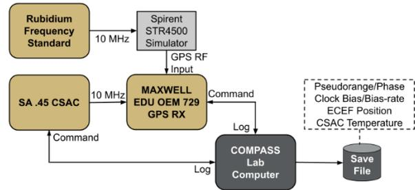
**Figure 7: Flight Mode Testing Setup**
