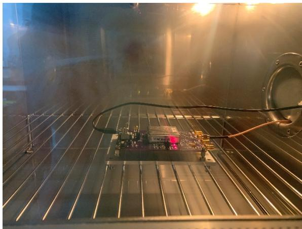
**Figure 9: CSAC Breakout Board Inside Thermal Chamber**
