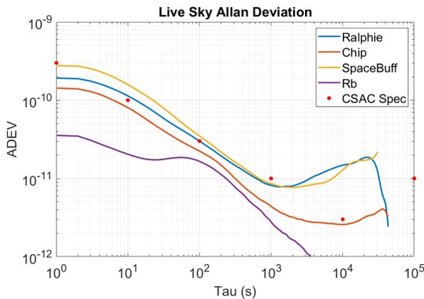
**Figure 3: Allan Deviation Using Receiver Estimated Clock Bias from CSAC and Rb Live Sky Tests**
