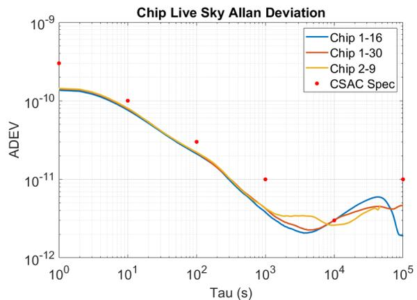
**Figure 4: Allan Deviation Using Receiver Estimated Clock Bias: Comparing *Chip* Live Sky Tests**
