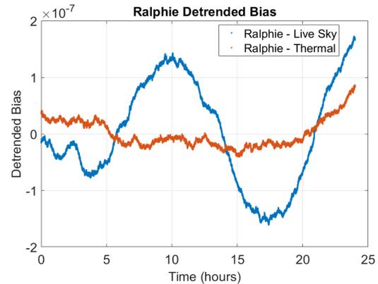
**Figure 11: Receiver Estimated Detrended Clock Bias of *Ralphie* Comparing Live Sky and Constant Temperature Hot Tests**
