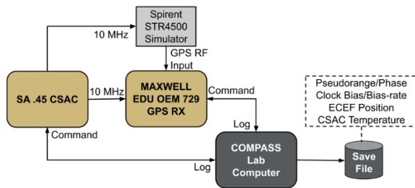
**Figure 5: Locked-Clock Testing Setup Using CSAC as External Reference to GPS Receiver and Spirent Simulator**
