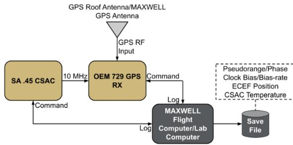
**Figure 1: Block Diagram of the Flight Configuration and Live Sky Testing Setup for the CSAC Experiment**
