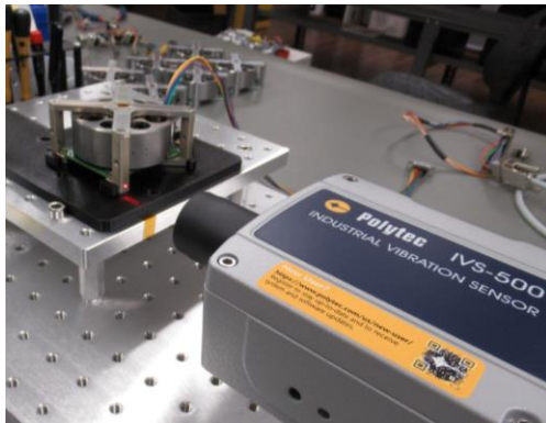
Figure 9: View of the RW-0.06 Product Placed on a Standoff in Line with the Laser Doppler Vibrometer
