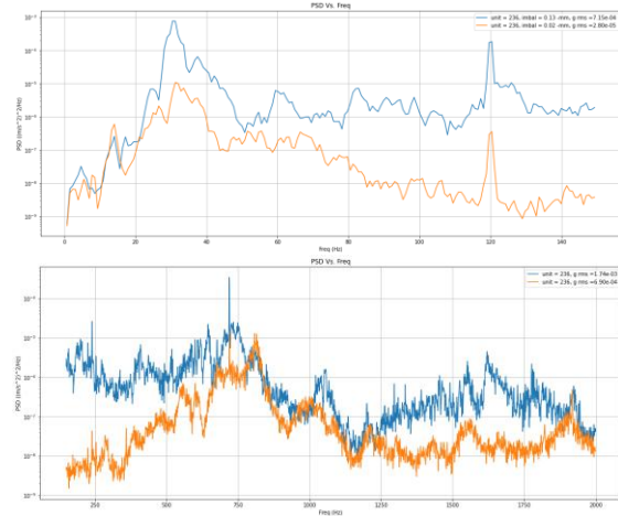
Figure 10: Low Frequency Range (top) and Medium Frequency Range (bottom). The Blue Line Indicates the System without Viscoelastic Dampers, and the Orange Line Indicates the System with Viscoelastic Dampers
