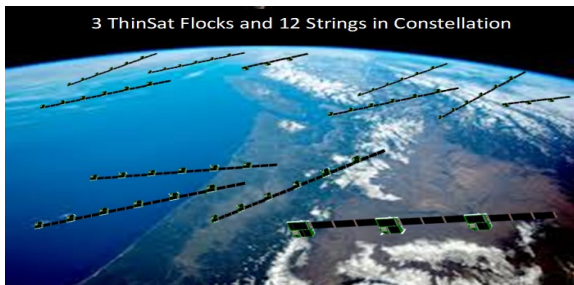
Figure 4 STRINGS: Educational Demonstration ThinSat Launch into a VLEO orbit on April 17, 2019 from Wallops Island, VA on NG-11 resupply ISS mission. Three 3U CSD launch containers each contained 21 ThinSats and 4 strings each for a total of 12 strings.
