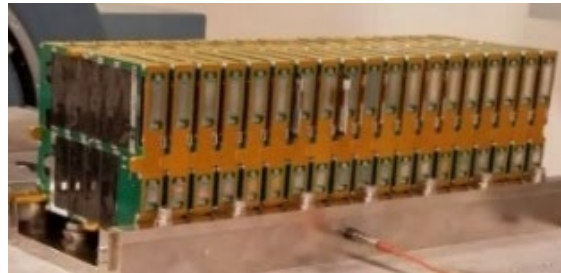
Figure 8 3U stack of 21 ThinSats mounted to a Test Fixture secured to the vibration table for testing. All three 3U CSDs passed testing for the Northrop Grumman Antares rocket.
