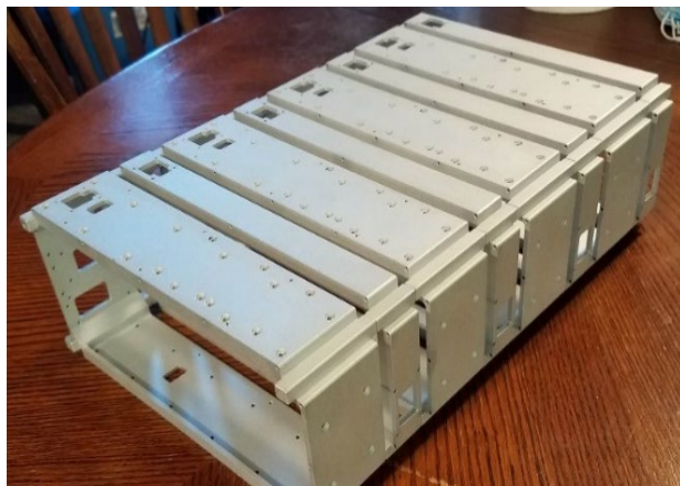
Figure 14 All 4 dual ThinSats compressed for loading into standard 2x3U launcher
