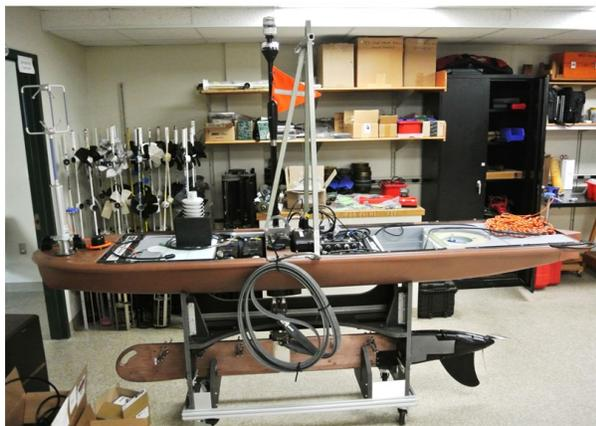
**Figure 3: Wave glider being prepped for deployment at WHOI. The sensors on the deck left to right include an Acoustic Doppler anemometer,**
