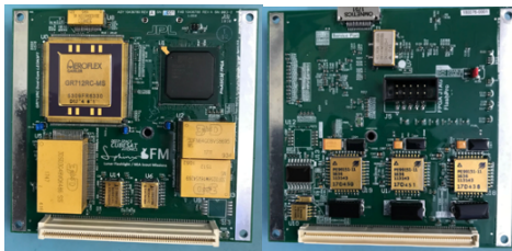
Figure 5: Sphinx FM PCB View (Top and Bottom)
