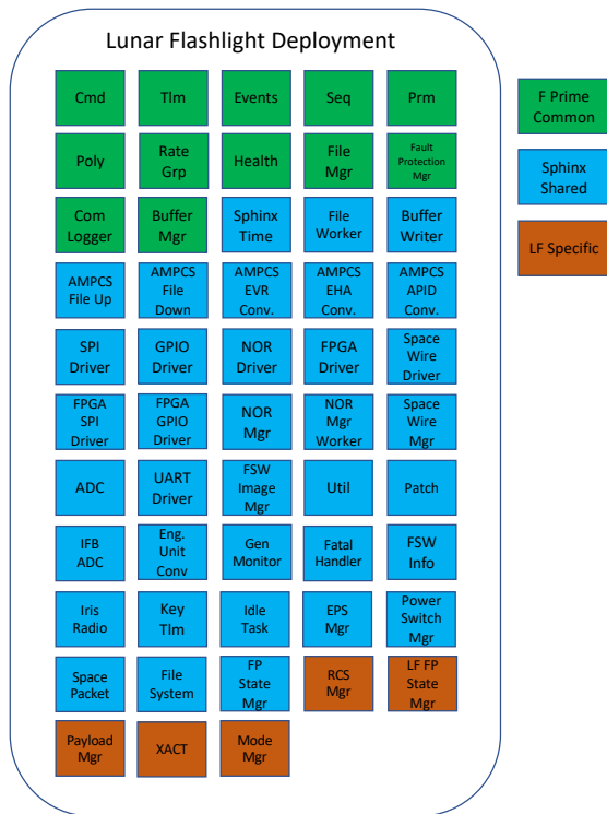
Figure 9: Lunar Flashlight Deployment Components
