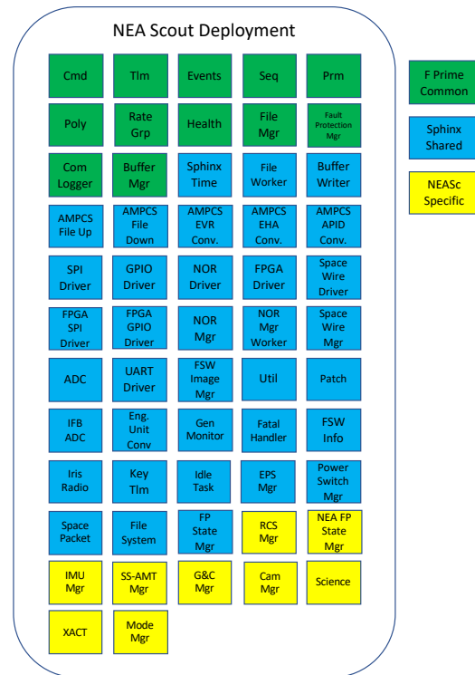
Figure 10: NEA Scout Deployment Components
