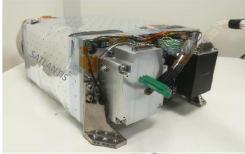
Figure 3: PM (Plane Model) opto-mechanics of iSIM-90 SWIR. The FM (Flight Model) will be slightly different, with a different VNIR detector
