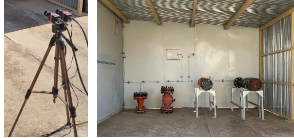
Figure 10: EM during validation campaign at ENAGÁS Zaragoza calibrated test bench
