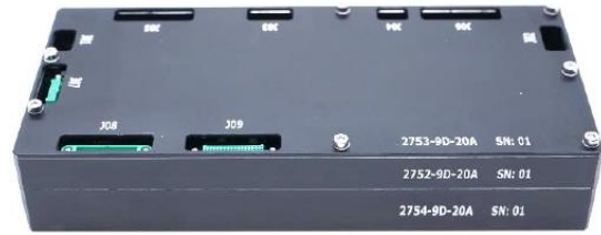
Figure 2: Electronic Control System box, with “SPoCK” PCB (for image acquisition and processing) and “Smart Heater” PCB of the Thermal Control System (for thermal stabilization) inside
