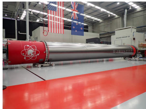
Figure 10: Silver Thermal Protection layer added to Electron first stage.
