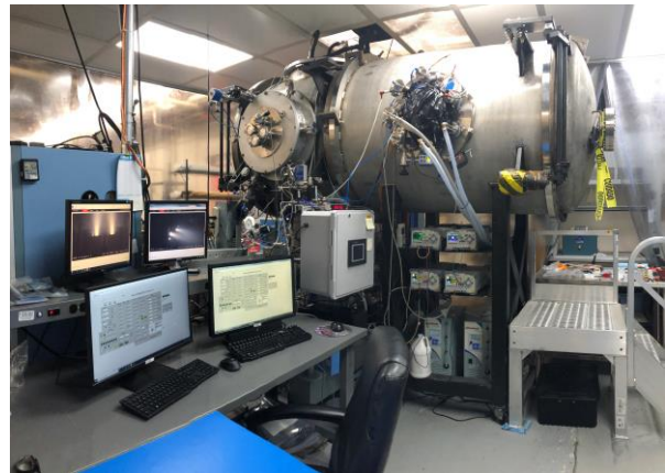
Figure 6: Busek's Upgraded T-4 Vacuum Facility
