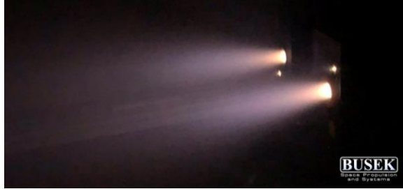
Figure 7: Twin Gen-2 BIT-3 Iodine Hot Firing
