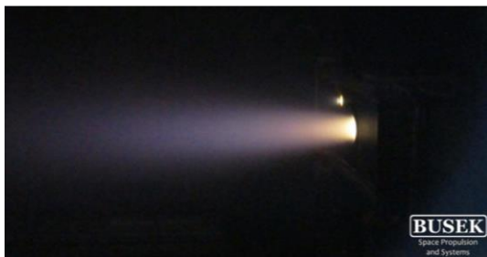
Figure 2: Gen-2 BIT-3 Iodine Hot Firing
