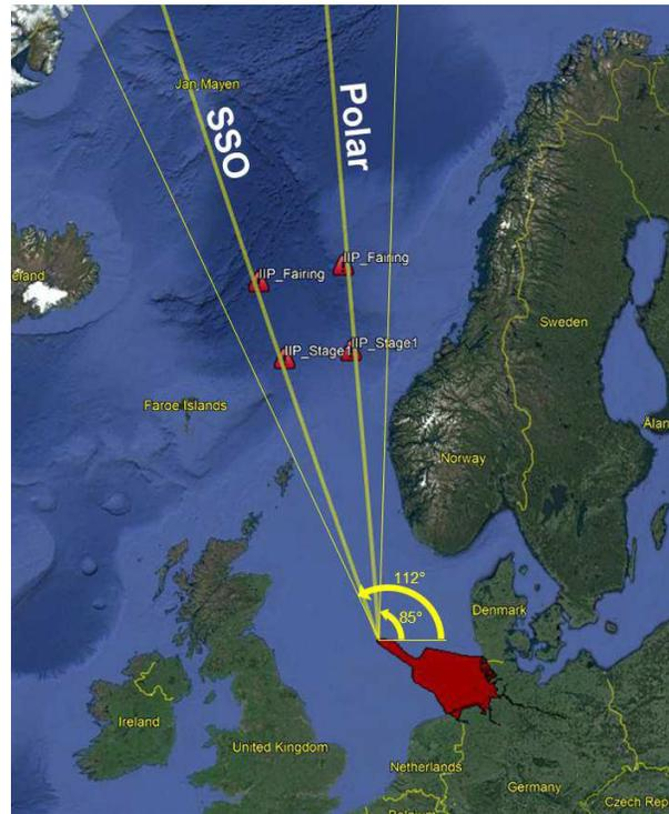
**Figure 1: Trajectory corridor of the planned offshore spaceport with a launch site in the German Exclusive Economic Zone (EEZ)**
