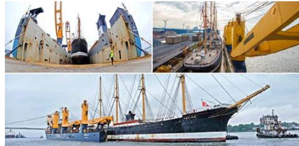
**Figure 3: Combi Dock RoRo Vessel, possible also to use as Flo Flo cargo transport (e.g. sailing ship)**
