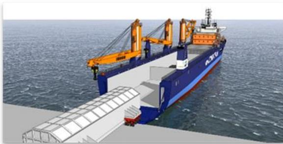
**Figure 5: Loading of the Mobile Launch Box in Roll-in-Roll-Out procedure**
