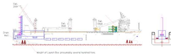
**Figure 6: Section view on Vessel and Launch Box during launch**
