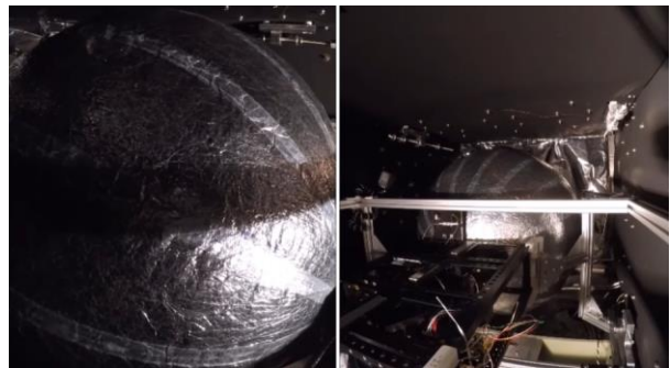
Figure 8: Inflatable antenna TVAC testing
