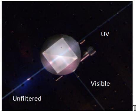
**Figure 4. Dichroic beam splitter for separating UV and optical wavelengths**
