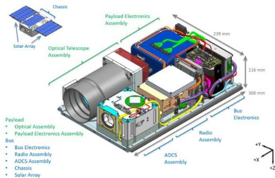
**Figure 6. Cutaway diagram showing optical telescope and subcomponents. (Credit Knapp 2019)**
