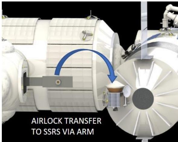
**Figure 6: Pressurized internal payloads can be transferred robotically to the awaiting SSRS using the airlock segment combined with the robotic arm.**
