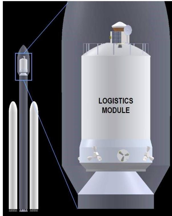
**Figure 3: Small spacecraft return system pathfinder concept externally attached to Logistics Module inside the launch vehicle 5.4 m diameter fairing.**
