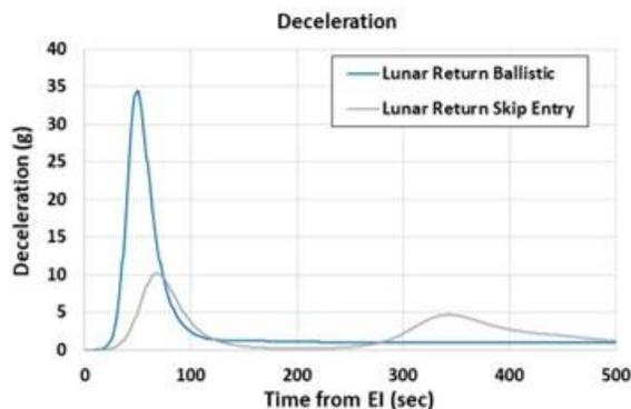
**Figure 9: Deceleration load comparison between ballistic and guided blunt body entry systems.**
