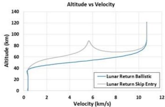
**Figure 7: Ballistic versus guided atmospheric flight trajectories from lunar return velocities, using a Stardust like ballistic vehicle (50 kg) entering with an entry flight path angle ( $\gamma$ ) of -6 deg with a guided blunt body capsule capable (70 deg, sphere cone, 1.5 m diameter, 100 kg entry mass) also entering at -6 deg  $\gamma$ , but with an angle of attack of -16 deg to generate lift.**
