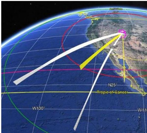
**Figure 8: Downrange comparison between the ballistic (yellow) and lifting (white) blunt body entry configurations.**
