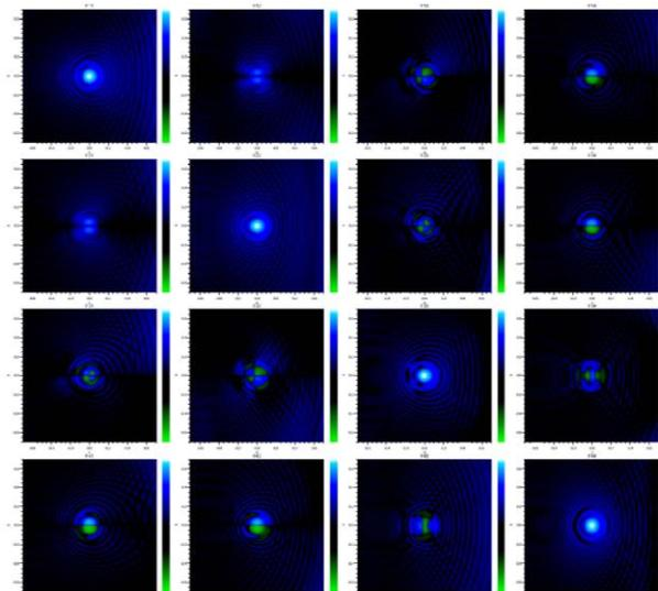
**Figure 4: Mueller matrix of the MEM antenna. The 4x4 matrix represents the co- and cross-pol antenna patters across all fourth Stokes parameters. The diagonal elements represent the co-pol. The color-scale has been normalized to 1 (white) and -1 (green).**
