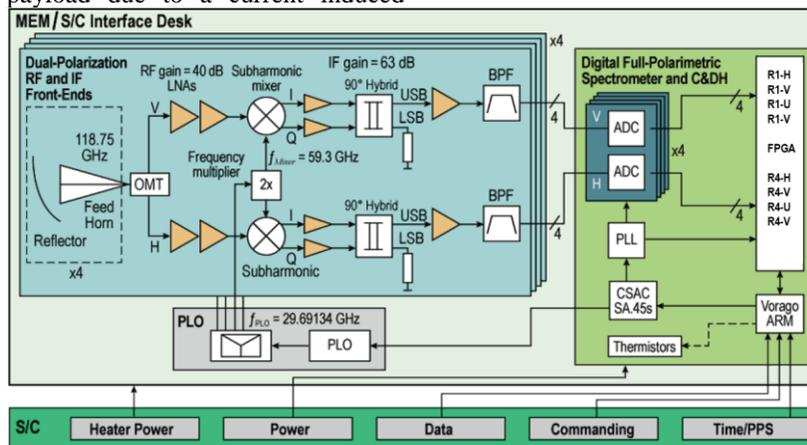
**Figure 2: Block-diagram of the MEM payload instrument**
