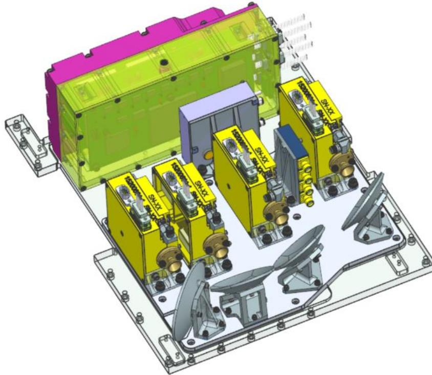
**Figure 3: CAD of the MEM payload instrument to be fit within a 2U system**
