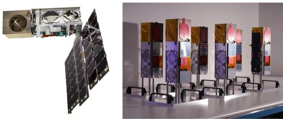
**Figure 1.** TROPICS satellite (left), showing the rotating payload connected to the satellite bus via a rotary joint. Also shown in the image on the left is the articulating solar array, which rotates (as does the satellite bus) to track the sun to maximize power output. The six satellites that will comprise the constellation are shown on the right. (Photo credit: Blue Canyon Technologies)
