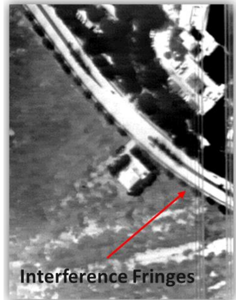
Figure 13: Lo Image of Oahu captured by a plane mounted prototype of the HyTi instrument 20
