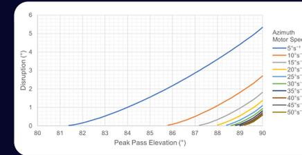
Figure 1. Maximum antenna pointing error arising from keyholing at different pass altitudes. Different azimuth motor speed curves are shown to illustrate the sensitivity of motor speed on the magnitude of keyholing.
