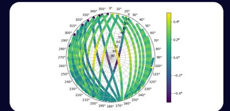
Figure 4. Azimuth-elevation diagram showing the difference between the motor-based encoder and an existing antenna encoder gathered from the ACU metrics. A periodicity of 10° can be seen in azimuth.
