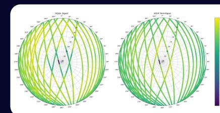
Figure 3. Relative received signal strengths for 37 Aqua satellite passes showing (left) received values, (right) normalised values adjusted for range and spacecraft antenna pattern.
