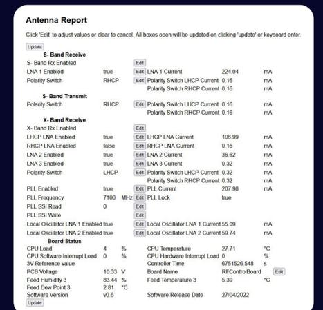
Figure 5. The ACU's current measurement metrics confirm the LNAs are nominal.
