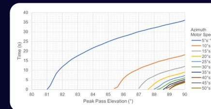
Figure 2. The amount of time the antenna needs to catch up with the spacecraft arising from keyholing at different pass altitudes. Different azimuth motor speed curves are shown to illustrate the sensitivity of motor speed on the time duration of keyholing.
