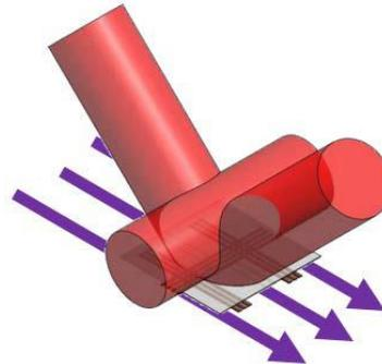
**Figure 2: Schematic of a mirror MOT, depicting the required laser beams (in red) and the macroscopic H wires. Purple arrows denote the direction of the required external, homogeneous, magnetic field (bias field).**
