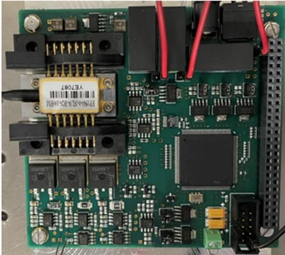
**Figure 3: Prototype seed laser package with a 14-pin butterfly mounted laser diode.**
