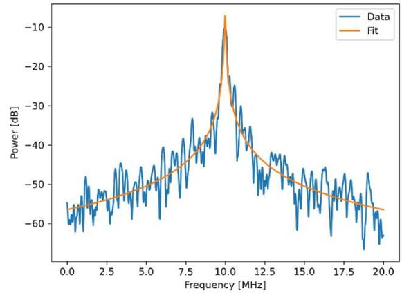
**Figure 4: Power spectrum of the beat note between a laser of know linewidth and CASPA ADM's seed laser**
