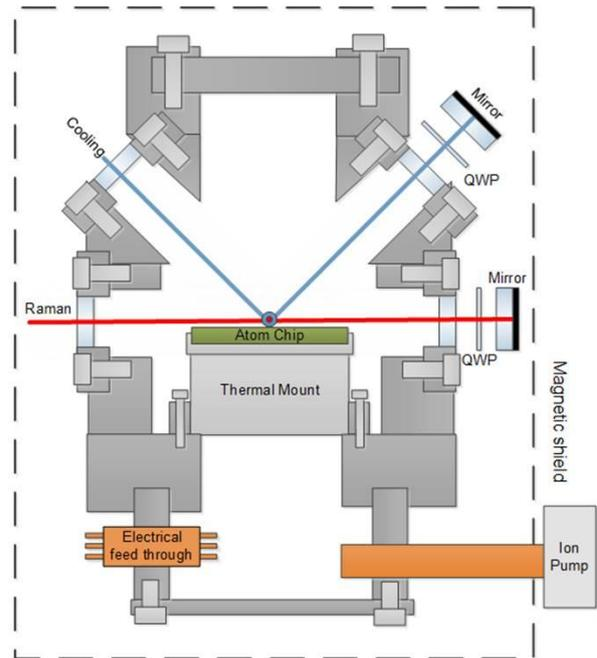
**Figure 6: Schematic of the physics package. Optical ports on the vacuum chamber allow access to Raman and cooling retro-reflected beams. An atom chip (RAL Space), together with a pair of external coils, generates the magnetic field required to trap the  $^{87}\text{Rb}$  atoms. A magnetic shield (dashed line) encloses the physics package.**
