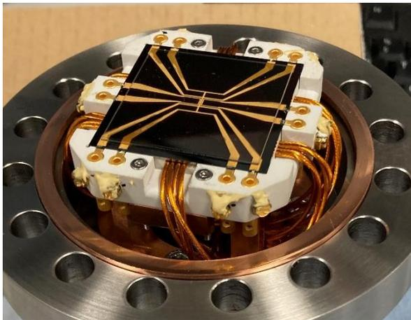
**Figure 1: Photograph of the second generation of atom chip developed at RAL Space (STFC-UKRI).**
