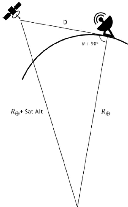
**Figure 5: Radio Link Geometry**
