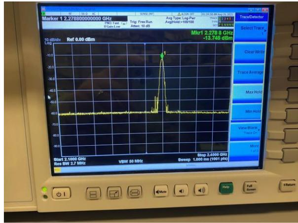
**Figure 3: Experimental Cadet Radio Signal Strength**
