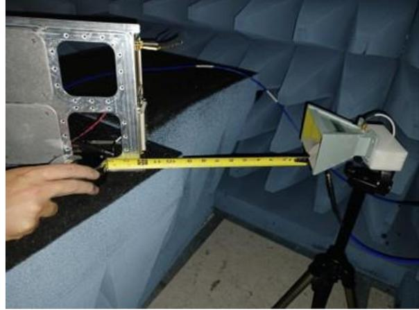
**Figure 2: Cadet Radio Signal Strength Test**
