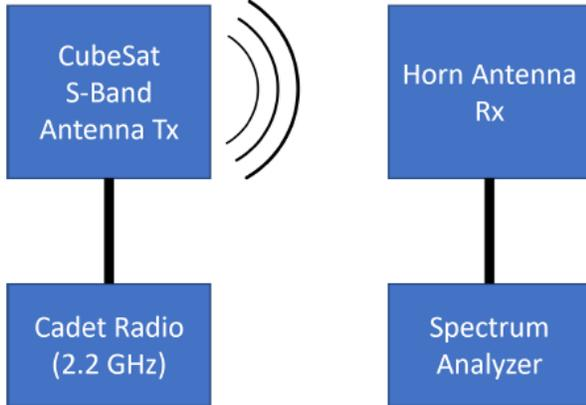
**Figure 1: Cadet Radio Signal Strength Test Setup Flow Chart**
