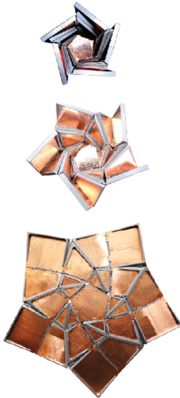
Figure 9: The flasher array's deployment process is illustrated with stowed, deploying, and fully deployed images. The full prototype unfolds from a small volume to span approximately 1 meter in diameter and provide 0.555\text{m}^2 of working optical area. Fresnel lenses may be replaced with thin copper plating (as shown in this image) for use as a reflectarray.
