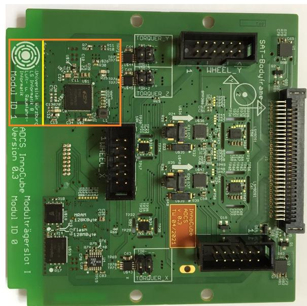
Figure 4: ADCS Board (SKITH marked orange)
