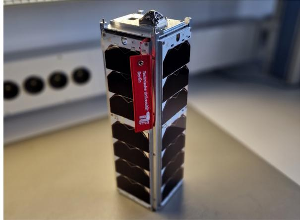
**Figure 1: InnoCube structural ground model**
