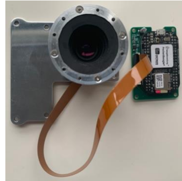
Figure 10, CROSS Engineering model for CUAVA-2.
