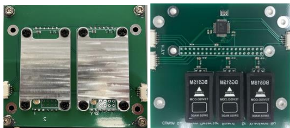
Figure 9 Engineering Model of Data over Power-bus (left) and Radiation Counter (right).
