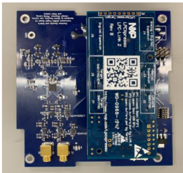
Figure 12, EDDI Engineering model for CUAVA-2
