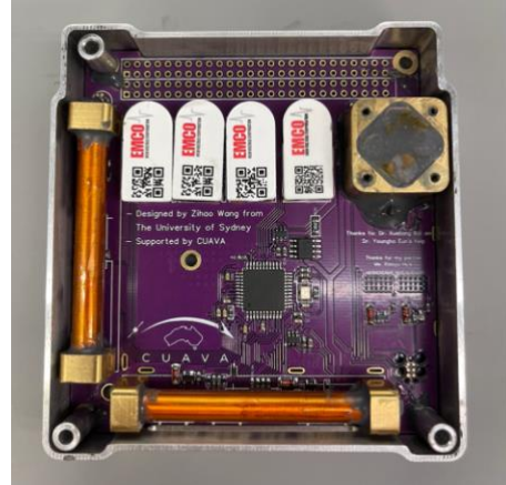
Figure 8: EPM Engineering model for CUAVA-2.
