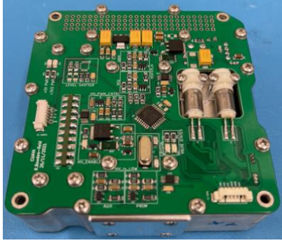
Figure 11, CXT Engineering model for CUAVA-2.
