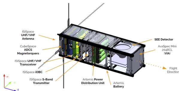
**Figure 5: Payload Location for VIA and SEE**
