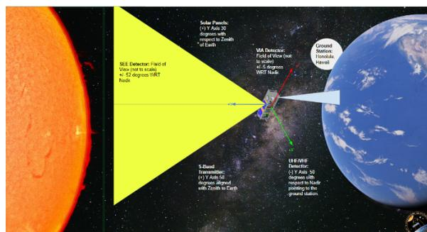
**Figure 1: Spacecraft Orientation and detector FOVs**
