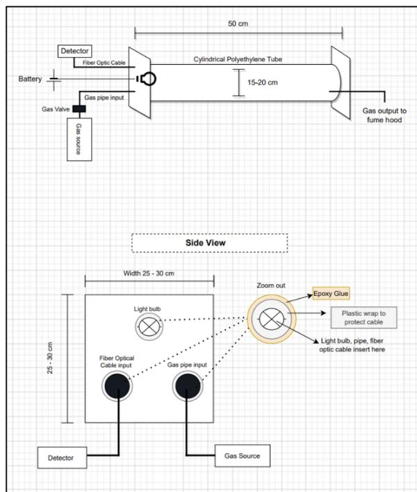
**Figure 4: Calibration chamber for VIA detector**
