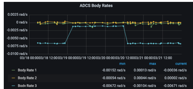
Figure 4: The spacecraft transition to fine point and the measured body rates as it went to fine point on March 19 th
