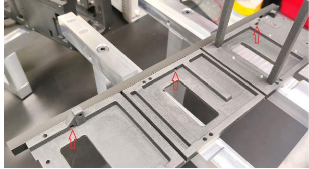
Figure 13: Locations of Aluminum Rail Fasteners to the Cover with Flat-Head Screws
