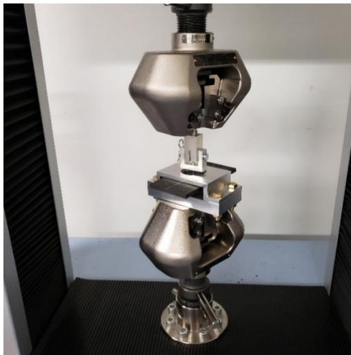
Figure 11: One of the Pull-Out Test Plates After Test (Left); Test Plate in CRP Test Fixture (Right)
