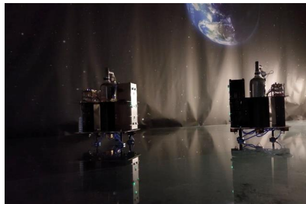
Figure 12: Testing Platform in 3Dof almost Frictionless Environment
