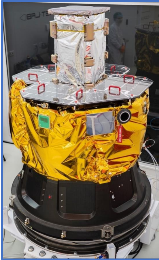
Figure 2: The CAPSTONE Spacecraft/Dispenser - Lunar Photon Integrated Stack
