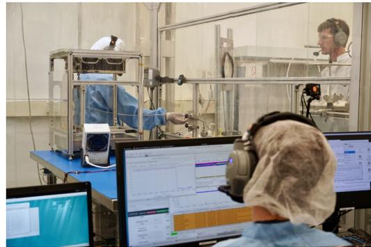
Figure 5: Propellant Loading Operation
