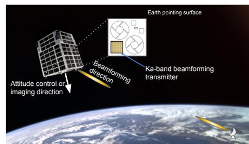
Figure 1: Illustration of AxelLink-Ka system
