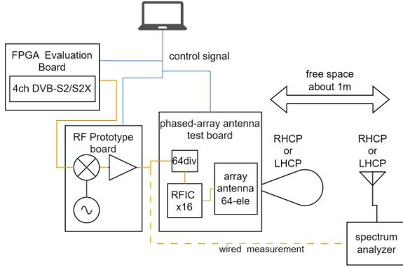
**Figure 6: Experimental setup for OTA**
