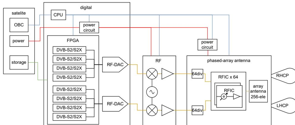
Figure 2: Block diagram of AxelLink-Ka transmitter
