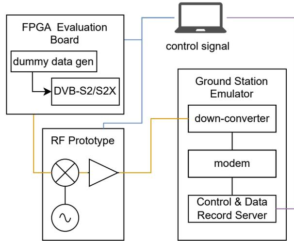
**Figure 8: Compatibility test with ground station emulator**
