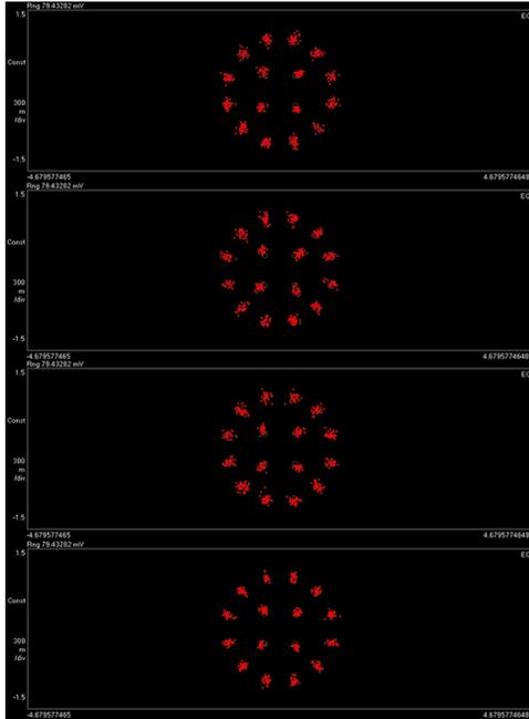
**Figure 7: Measured constellation for each multicarrier**
