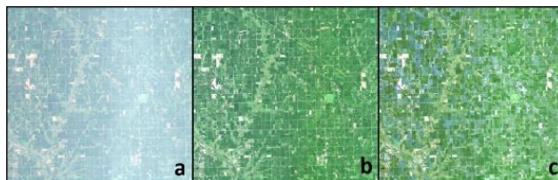
Figure 9. A view of the 8-11-18 L8 tile near Sioux Falls, SD affected by Canada wildfire smoke: (a) TOAR (b) corrected by CMAC; and (c) LaSRC with color balance issues.
