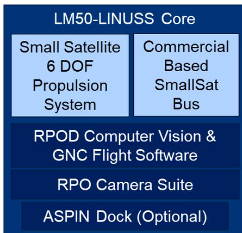
**Figure 3: Architecture block diagram of LM50-LM LINUSS core showing necessary integration of both RPO camera suite and flight software to ensure success of highly dependent subsystems.**
