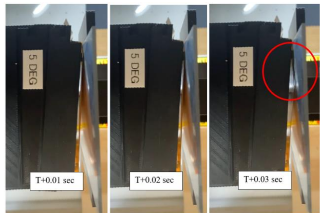
Figure 11: Attachment occurs faster for conductive materials.
