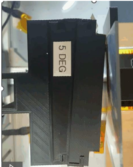
Figure 13: eTAP contact area with satellite mass simulator reduced to approximately 60% at 5° offset angle.
