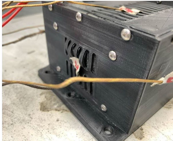
Figure 15: Thermal Distortion on Side Vent
