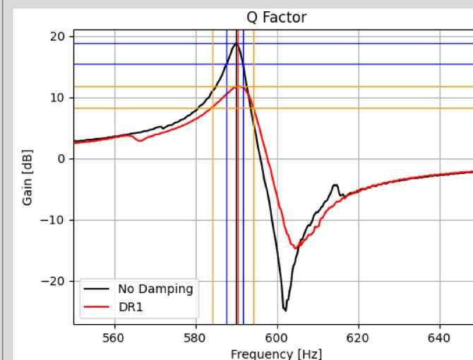
Applying these formulas to the responses of the undamped rotor and DR1 yields following values. Comparing the Q-factors, the CLD approach lowered the Q-factor by 59,2%. When comparing resonance frequencies, no significant shift is observed. This in combination with the fact that the material, shape and mass remained the same, allows us to conclude that CLD provided a way to increase the damping of the rotor while leaving its stiffness untouched.
