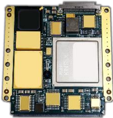
Figure 5: SpaceCube v3.0 Mini 1U Kintex UltraScale CubeSat Single-Board Computer Primary Side
