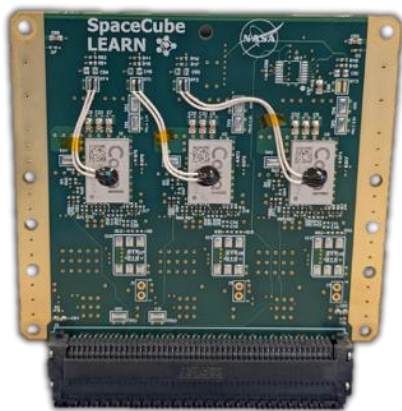
Figure 7: SpaceCube Low-power Edge Artificial Intelligence Resilient Node (SC-LEARN) with Thermistors Populated
